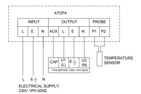
Output connections from controller to fan motor
