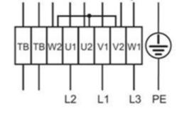
$\begin{array}{ll} \mbox{High speed} & \mbox{Low Speed} \\ \mbox{$\Delta$-Connection} & \mbox{Y-Connection} \end{array}$
