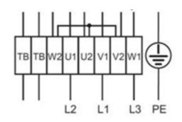
High speed Low Speed Δ-Connection Y-Connection
