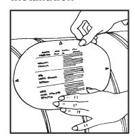
1. Stick self adhesive template on to duct (a template is provided with each door).
