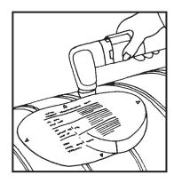
2. Cut out aperture (there is a tolerance of +3mm).
