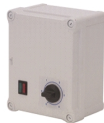
Auto-transformer. Single phase 230V-50 Hz. Wall mounting. IP44. Motor PTO connection. Maximum switch output: (1A).
