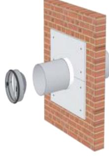
Insert damper in the duct
