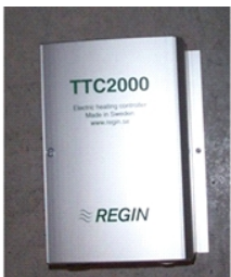
ELECTRICAL HEATER BATTERY CONTROLLER
