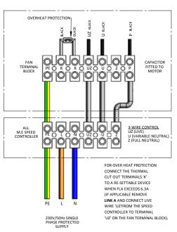
FAN CONNECTED TO SUPPLY (FULL SPEED)
