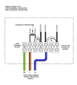
FAN CONNECTED TO SUPPLY (FULL SPEED)
