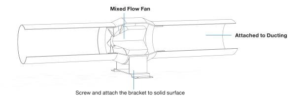
The use of Fast Clamps or Flexible Connectors is recommended for connection to duct, making it very easy for future maintenance, repair, or replacement.
