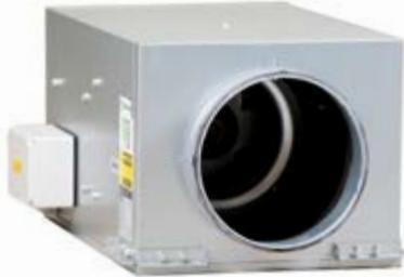
**Acoustically lined single in-line centrifugal fans, suitable for internal duct mounting. The Quietflow incorporates advanced backward curved impellers, with three dimensional profiled blades.**
