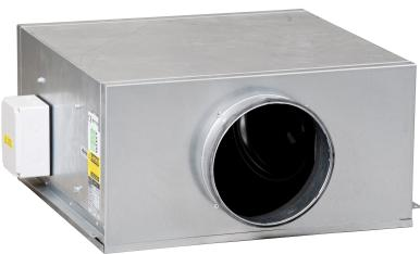
**The Quietflow SQT fans are acoustically lined twin in-line centrifugal fans, suitable for internal duct mounting. The Quietflow incorporates advanced backward curved impellers, with three dimensional profiled blades.**
