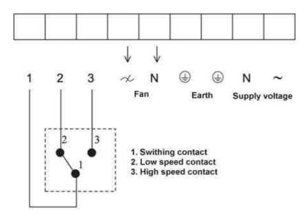
NB A swithing contact has to be connected
