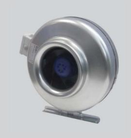
The SDX Euroflow in-line centrifugal duct fans are designed around an efficient backward curved centrifugal impeller and external rotor motor to ensure a compact design, high performance and low sound levels.
