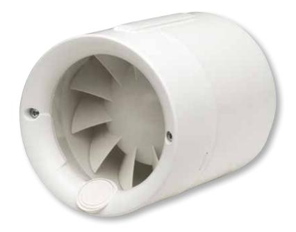
Transfer axial fan offering a very low noise level and specifically designed to work through a duct or to be flush mounted into the wall, ideal for ventilating small areas or to exchange heat between adjoining rooms. Fitted with single phase motors 230V-50Hz, IP44, Class II, with ball bearings for enhanced working life and assembled on silent-blocks.
