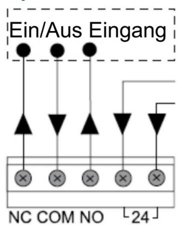
Power supply: 24V AC/DC (non-polarity)
