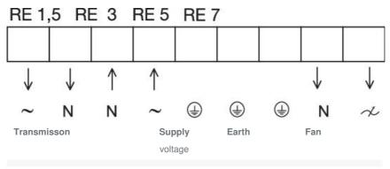
Transmisson:between ~ and N is always 230V when the transformer handle is in pos. 1-5
