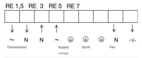
Transmisson:between  $\sim$  and N is always 230V when the transformer handle is in pos. 1-5
