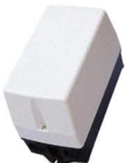
9A 2 x N/O / 2 x N/C relay in IP65 enclosure for switching of fans from an external source.
