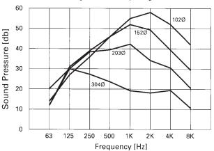
**Note:** Care should be taken when estimating the attenuation of ducts of different lengths; the results are not linear. The possibility of noise 'break-out' should also be taken into consideration at the design stage since there may be some noise emission into the surrounding air space. Wherever possible acoustic ducting should be installed in a part of the building where noise break-out is not of concern or above an acoustic/insulated ceiling to prevent noise reaching the occupied areas.
