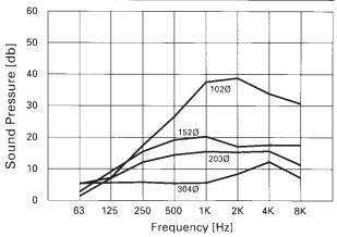
Static Insertion Loss measurements - 3 metre length
