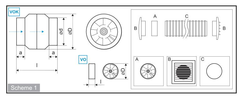
All VO and VOK series fans can be produced with length "I" to suit most specific requirements of our customers. The length "I" for the VO series indicated in the tables below is the minimum length possible to achieve.
