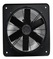
• Frame with port and grille made of pressed steel, pickled and phosphated, and treated initially with epoxy base coat; thereafter, grey textured finish obtained by applying a coat of polyurethane powder paint strengthened by oven baking.
