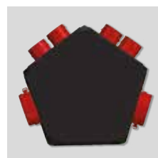
PLENUM UNI EX 5P/125 Insulated extraction plenum of 125mm diameter, 1 Kitchen spigot of 125mm diameter and 4 sanitary spigots of 80mm diameter.
