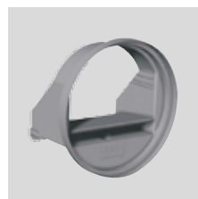
RD BP Specific low-pressure (20-100 Pa) and self-adjusting damper with sleeve to fit directly into the duct. 80mm diameter. Airflow: 15 or 30 m³/h.
