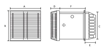
Wall fixing hole 250mm x 250mm sq.
