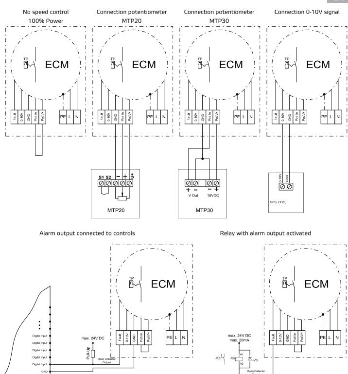
An open-collector output is a digital low-voltage output in which the height voltage for the signal is applied via a pull-up resistor. If the pull-up is supplied with 5 Vdc, the high level is 5V and the low level is 0V
