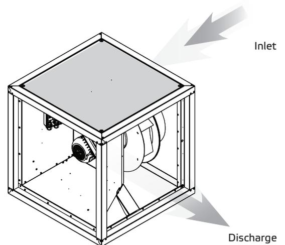
By closing an open side, the discharge side can be changed.
