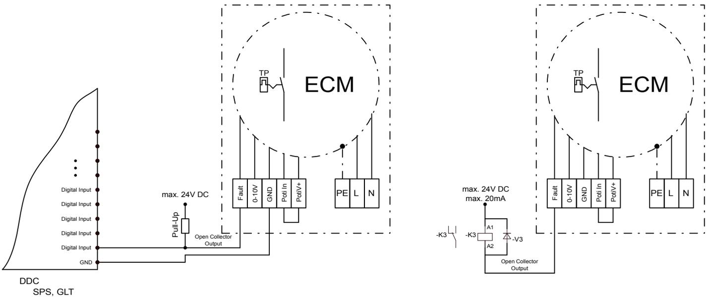
An open-collector output is a digital low-voltage output in which the height voltage for the signal is applied via a pull-up resistor. If the pull-up is supplied with 5 Vdc, the high level is 5V and the low level is 0V
